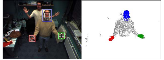
Fig. 4. Left: camera image (rectangle: head, circle: hand1, cross: hand2). Right: observations assigned to one of the four models depending on their probabilities (blue: head, red: hand1, green: hand2, grey: discard, white: pixels ignored in EM).
